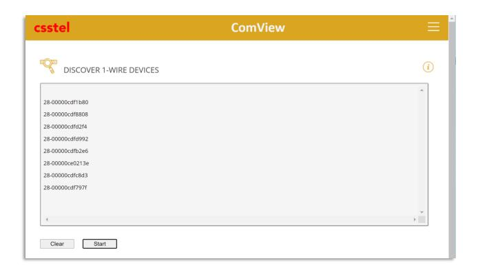
The values shown are the 8 IDs of DS18B20 1-Wire devices connected to the 1-Wire port of ComView and detected by the utility.
